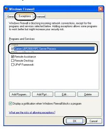
• If you installed the CAPT software by any method other than CD-ROM Setup, you need to use the CAPT Windows Firewall Utility software to configure Windows Firewall to unblock communication with the client computers. (See p. 7-8)
